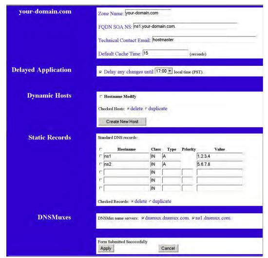
If making changes to an existing zone, the zone name is shown in the upper left. If setting up a new zone, "New Zone" is shown.
