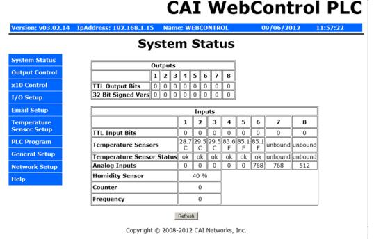
Figure 3.0 WebControl<sup>TM</sup> PLC system status
