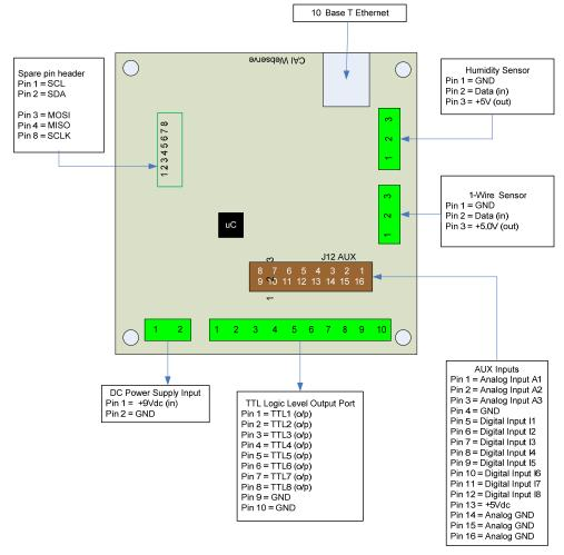
Figure 1.0 WebControl<sup>™</sup> PCB inputs and outputs diagram
