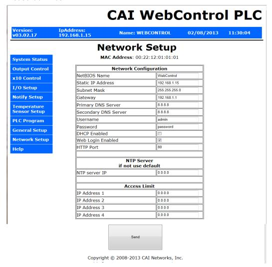
Figure 4.0 WebControl<sup>TM</sup> PLC Network configurable
