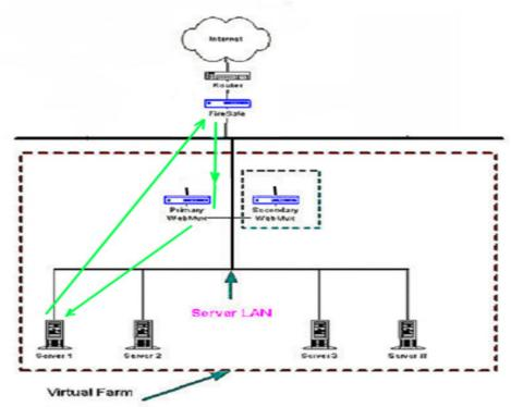
In most situations, the incoming traffic is in small requests, and return traffic from servers back to clients is large amount of data, pictures, or documents. Using direct routing will allow up to 100 times more traffic to be handled by the WebMux load balancer. The disadvantage for direct routing is that the firewall protections built-in to WebMux will no longer function. Users then must provide their own firewall for incoming and outgoing traffic.
