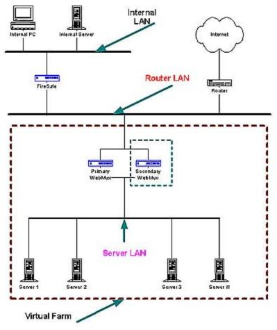
The main purpose of the WebMux is to balance the traffic among multiple web or other servers. The diagram above shows an NAT installation with two WebMuxes. In this configuration, one WebMux is serving as the primary, and the other is serving as the secondary, or backup, providing a fault tolerant solution.
