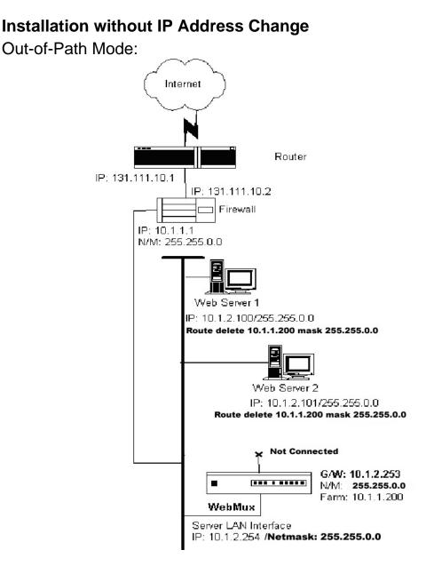
The above diagram is an example about how to configure the WebMux in out-ofpath mode without changing the IP addresses of the web servers and other servers that already exist on the network. This is particularly helpful when the changing of an existing network of servers causes problems.
