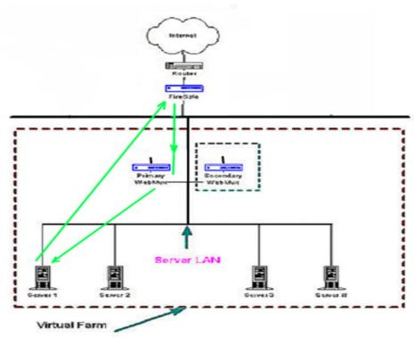
In most situations, the incoming traffic is in small requests, and return traffic from servers back to clients is large amount of data, pictures, or documents. Using direct routing will allow up to 100 times more traffic to be handled by the WebMux load balancer. The disadvantage for direct routing is that the firewall protections built-in to WebMux will no longer function. Users then must provide their own firewall for incoming and outgoing traffic.
