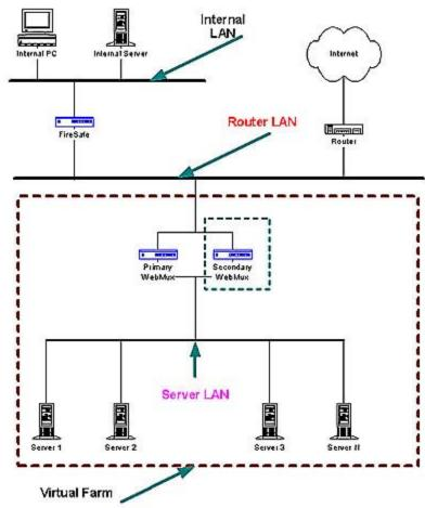
The main purpose of the WebMux is to balance the traffic among multiple web or other servers. The diagram above shows an NAT installation with two WebMuxes. In this configuration, one WebMux is serving as the primary, and the other is serving as the secondary, or backup, providing a fault tolerant solution.
