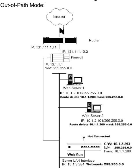
The above diagram is an example about how to configure the WebMux in out-of-path mode without changing the IP addresses of the web servers and other servers that already exist on the network. This is particularly helpful when the changing of an existing network of servers causes problems.
