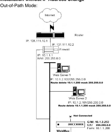
The above diagram is an example about how to configure the WebMux<sup>™</sup> in outof-path mode without changing the IP addresses of the web servers and other servers that already exist on the network. This is particularly helpful when the changing of an existing network of servers causes problems.
