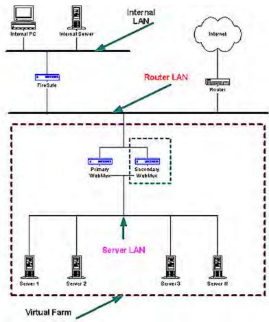
The main purpose of the WebMux<sup>™</sup> is to balance the traffic among multiple web or other servers. The diagram above shows an NAT installation with two WebMuxes. In this configuration, one WebMux<sup>™</sup> is serving as the primary, and the other is serving as the secondary, or backup, providing a fault tolerant solution.
