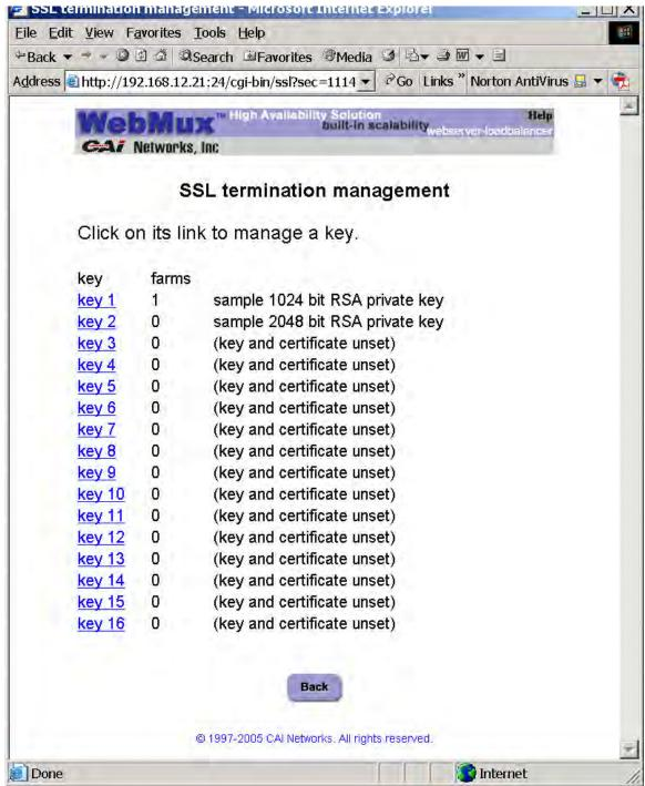
WebMux<sup>™</sup> model 480S, 580SG, 680PG support SSL termination. For models that do not support SSL termination, please ignore this section. WebMux<sup>™</sup> supports SSL V2, SSL V3, and TLS V1 with RSA key length from 512, 1024, and 2048.
