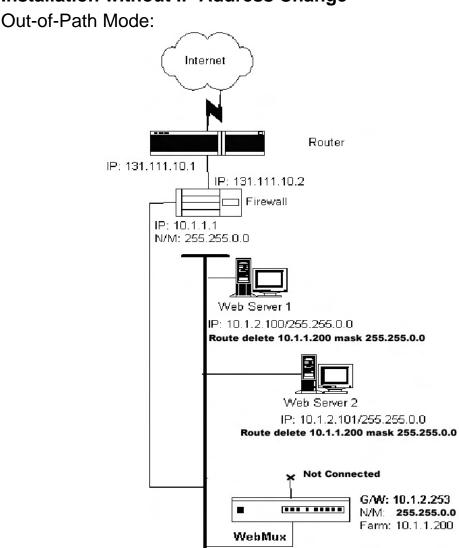
The above diagram is an example about how to configure the WebMux<sup>™</sup> in outof-path mode without changing the IP addresses of the web servers and other servers that already exist on the network. This is particularly helpful when the changing of an existing network of servers causes problems.
