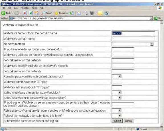
When the mouse moved over a field, the current value will be automatically filled. The user may change it based on new information obtained from ISP or network engineers. Once you press on the submit button, the WebMux<sup>™</sup> will save all the changes to its internal solid state storage and reboot itself with the new value.
