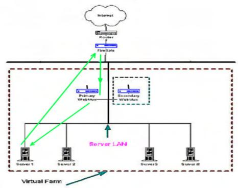
In most situations, the incoming traffic is in small requests, and return traffic from servers back to clients is large amount of data, pictures, or documents. Using direct routing will allow up to 100 times more traffic to be handled by the WebMux<sup>™</sup> load balancer. The disadvantage for direct routing is that the firewall protections built-in to the WebMux™ will no longer function. Users then must provide their own firewall for incoming and outgoing traffic.
