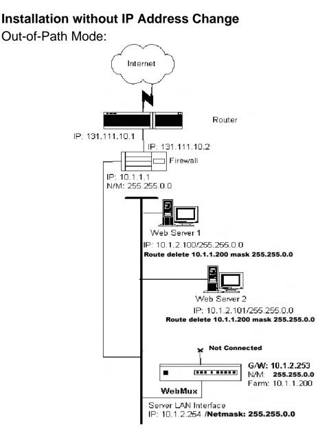
The above diagram is an example about how to configure the WebMux<sup>™</sup> in outof-path mode without changing the IP addresses of the web servers and other servers that already exist on the network. This is particularly helpful when the changing of an existing network of servers causes problems.
