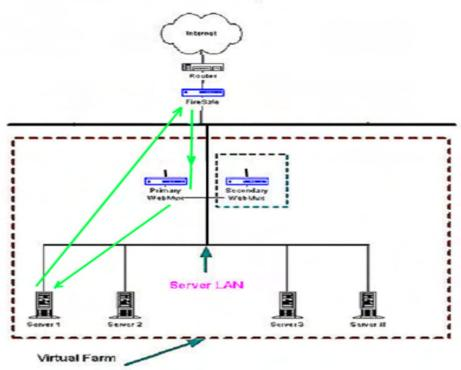
In most situations, the incoming traffic is in small requests, and return traffic from servers back to clients is large amount of data, pictures, or documents. Using direct routing will allow up to 100 times more traffic to be handled by the WebMux<sup>™</sup> load balancer. The disadvantage for direct routing is that the firewall protections built-in to the WebMux<sup>™</sup> will no longer function. Users then must provide their own firewall for incoming and outgoing traffic.
