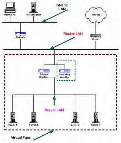
The main purpose of the WebMux<sup>TM</sup> is to balance the traffic among multiple web or other servers. The diagram above shows an NAT installation with two WebMuxes. In this configuration, one WebMux<sup>TM</sup> is serving as the primary, and the other is serving as the secondary, or backup, providing a fault tolerant solution.
