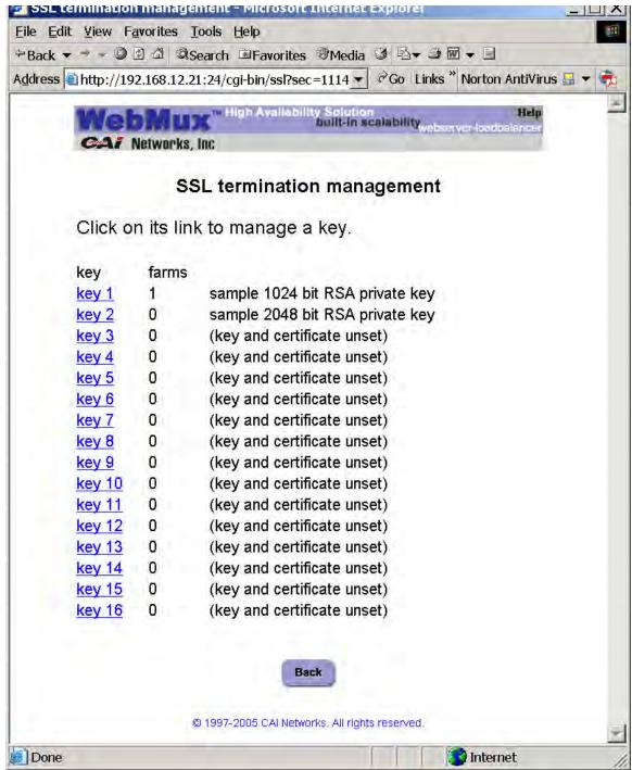
WebMux<sup>™</sup> model 481S, 591SG, 680PG support SSL termination. For models that do not support SSL termination, please ignore this section. WebMux<sup>™</sup> supports SSL V2, SSL V3, and TLS V1 with RSA key length from 512, 1024, and 2048. For each WebMux<sup>™</sup>, one can have 16 SSL certificates: Any key can be active or not active. The first line of the private key is the comment. See included
