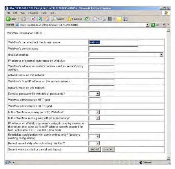
When the mouse moved over a field, the current value will be automatically filled. The user may change it based on new information obtained from ISP or network engineers. Once you press on the submit button, the WebMux<sup>™</sup> will save all the changes to its internal solid state storage and reboot itself with the new value.
