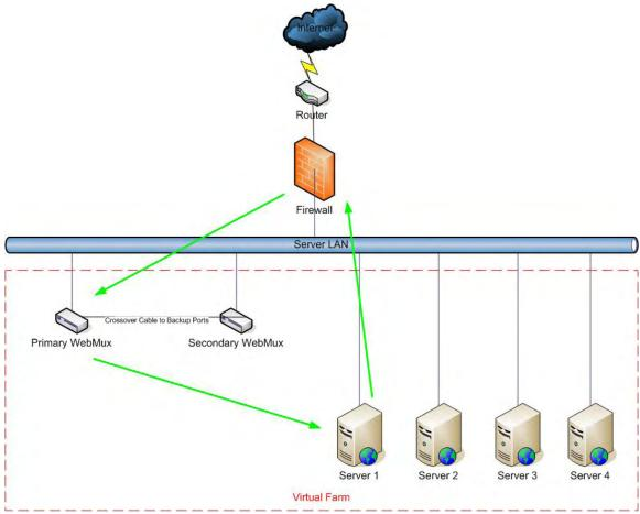
In most situations, the incoming traffic is in small requests, and return traffic from servers back to clients is large amount of data, pictures, or documents. Using out-of-path mode will allow up to 100 times more traffic to be handled by the
