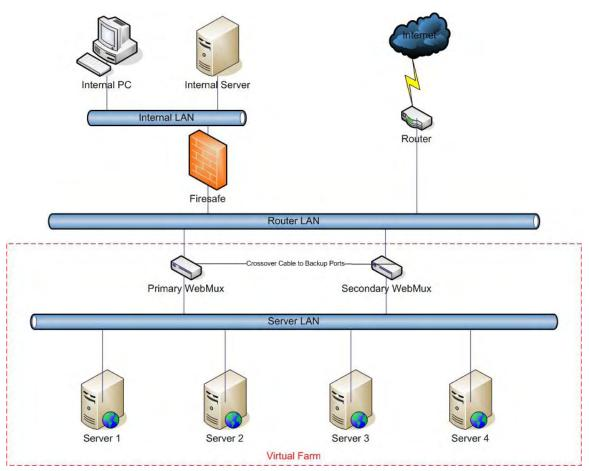
The main purpose of the WebMux<sup>™</sup> is to balance the traffic among multiple web or other servers. The diagram above shows an NAT installation with two WebMuxes. In this configuration, one WebMux<sup>™</sup> is serving as the primary, and the other is serving as the secondary, or backup, providing a fault tolerant solution.
