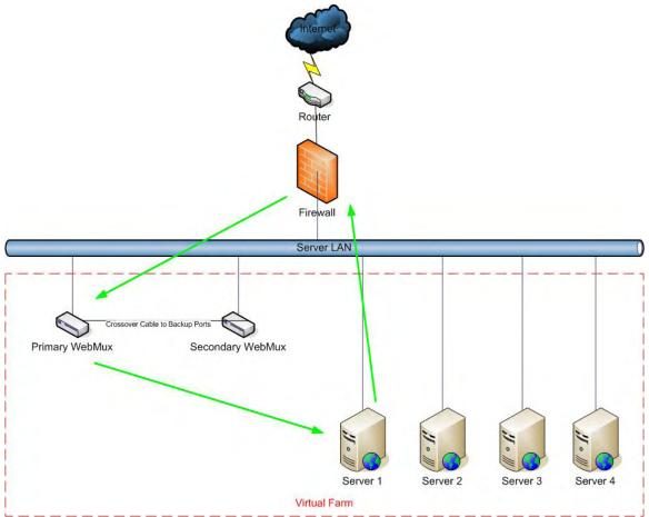
In most situations, the incoming traffic is in small requests, and return traffic from servers back to clients is large amount of data, pictures, or documents. Using out-of-path mode will allow up to 100 times more traffic to be handled by the WebMux<sup>™</sup> load balancer. The disadvantage for OOP/direct responding is that the firewall protections built-in to the WebMux<sup>™</sup> will no longer function. Users then must provide their own firewall for incoming and outgoing traffic.
