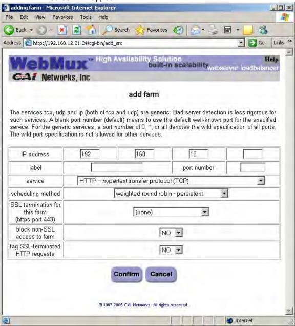
By default, the SSL termination is NOT on. The description here is for for the 481S model. Other models can be configured similarly.
