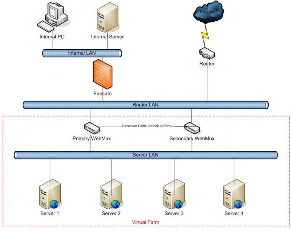
The main purpose of the WebMux<sup>™</sup> is to balance the traffic among multiple web or other servers. The diagram above shows an NAT installation with two WebMuxes. In this configuration, one WebMux<sup>™</sup> is serving as the primary, and the other is serving as the secondary, or backup, providing a fault tolerant solution.
