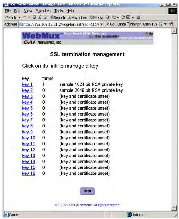
WebMux<sup>™</sup> model 481S, 591SG, 680PG support SSL termination. For models that do not support SSL termination, please ignore this section. WebMux<sup>™</sup> supports SSL V2, SSL V3, and TLS V1 with RSA key length from 512, 1024, and 2048. For each WebMux<sup>™</sup>, one can have 32 SSL certificates: Any key can be active or not active. The first line of the private key is the comment. See included
