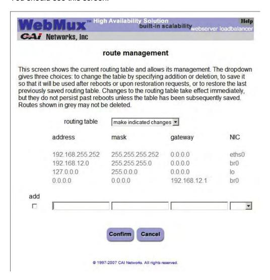
Routes displayed that are "grayed out" cannot be modified. To add a route, make sure "make indicated changes" is selected in the drop down menu, click the "add" checkbox, and fill in the remaining fields. Click the "confirm" button. Your new route should appear along with a "delete" checkbox. You can click on
