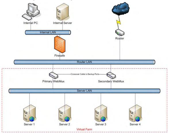
The main purpose of the WebMux™ is to balance the traffic among multiple web The diagram above shows an NAT installation with two or other servers. WebMuxes. In this configuration, one WebMux™ is serving as the primary, and the other is serving as the secondary, or backup, providing a fault tolerant solution.
