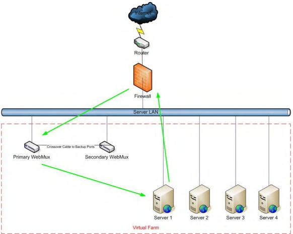
In most situations, the incoming traffic is in small requests, and return traffic from servers back to clients is large amount of data, pictures, or documents. Using out-of-path mode will allow up to 100 times more traffic to be handled by the WebMux<sup>™</sup> load balancer. The disadvantage for OOP/direct response is that the
