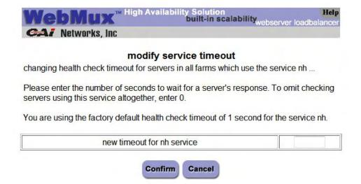
The setting in this page will determine how long or how short the WebMux will wait to be able to verify if the gateway IP is still valid or not. You can disable the checking altogether by setting the timeout value to 0 or you can set the "front network verification" protocol to "none" in the Administrator Setup page (see Section 6.3).
