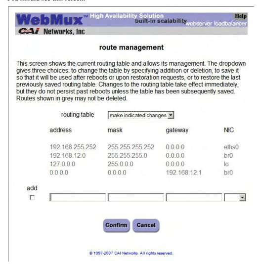
Routes displayed that are "grayed out" cannot be modified. To add a route, make sure "make indicated changes" is selected in the drop down menu, click the "add" checkbox, and fill in the remaining fields. Click the "confirm" button. Your new route should appear along with a "delete" checkbox. You can click on the "delete" checkbox and click confirm to delete the selected route. Please remember that even though a new route is immediately active once you
