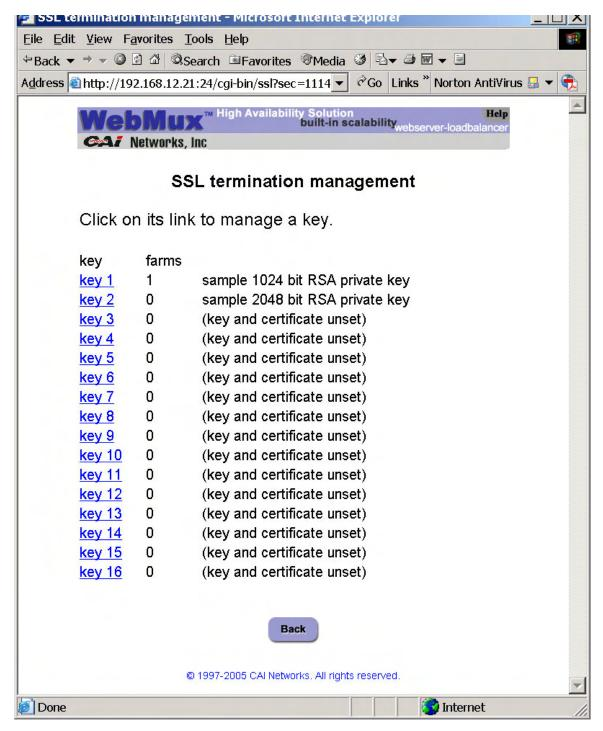
The WebMux supports SSL V2, SSL V3, and TLS V1 with RSA key length from 512, 1024, and 2048. For each WebMux, one can have 32 SSL certificates: Any key can be active or not active. The first line of the private key is the comment. See included two sample keys for
