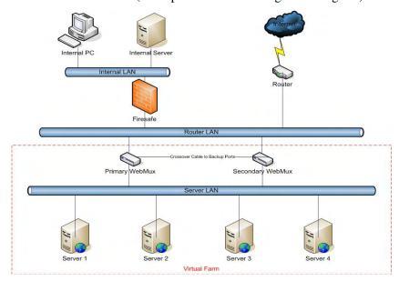
The main purpose of the WebMux is to balance the traffic among multiple web or other servers. The diagram above shows a NAT installation with two WebMuxes. In this configuration, one WebMux is serving as the primary, and the other is serving as the secondary, or backup, providing a fault tolerant solution.
