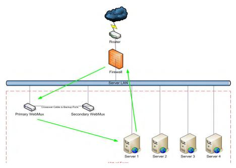
In most situations, the incoming traffic is in small requests, and return traffic from servers back to clients is large amount of data, pictures, or documents. Using out-of-path mode will allow up to 100 times more traffic to be handled by the WebMux load balancer. The disadvantage for OOP/direct response is that the firewall protections built-in to the WebMux will no longer function. Users must provide their own firewall for incoming and outgoing traffic.
