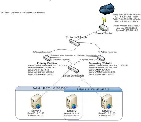
• The installation requires two WebMuxes. One will be the primary, and the other the secondary. They connect together with the Ethernet cable that is either cross-over or through a hub or switch. The primary's Backup interface IP address is 192.168.255.253; the secondary's Backup interface IP address is 192.168.255.254. They cannot be changed.
