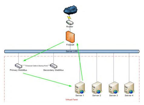
In most situations, the incoming traffic is in small requests, and return traffic from servers back to clients is large amount of data, pictures, or documents. Using Out-of-Path Mode will allow up to 100 times more traffic to be handled by the WebMux load balancer. The disadvantage for OOP/direct response is that the firewall protections built-in to the WebMux will no longer function. Users must provide their own firewall for incoming and outgoing traffic.
