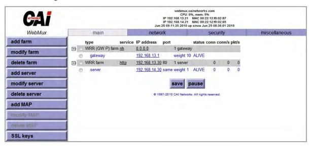
Your original default external gateway will be automatically added to the nexthop gateway farm. Click on the nexthop gateway farm IP on the grey line above the router IP to add more gateways to the nexthop farm.
