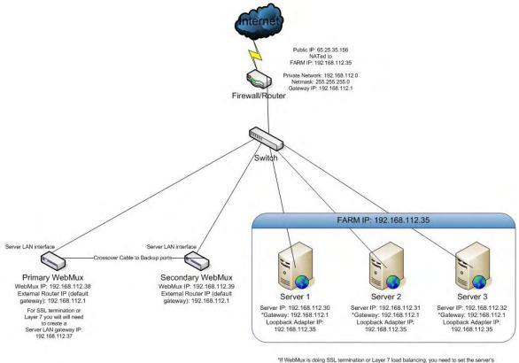
\*If WebMux is doing SSL termination or Layer 7 load balancing, you need to set the server's default gateway IP to the WebMux Server LAN gateway IP: 192.168.112.37
