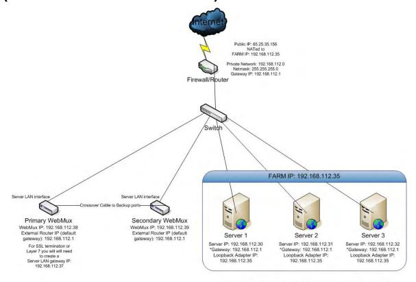
"If WebMux is doing SSL termination or Layer 7 load balancing, you need to set the server's default gateway IP to the WebMux Server LAN gateway IP: 19.21.68.112.37
