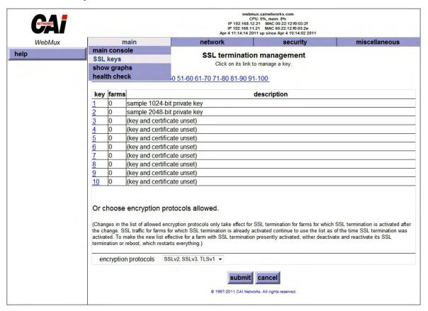
The WebMux supports SSL V2, SSL V3, and TLS V1 with RSA key length from 512, 1024, and 2048. For each WebMux, one can have 32 SSL certificates: Any key can be active or not active. The first line of the private key is the comment. See included two sample keys for details. If there is no comment line in the key, it will be blank. If there is no key, it will display "(key and certificate unset)."
