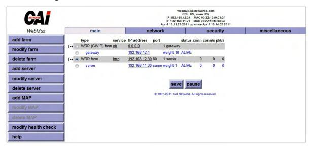
Your original default external gateway will be automatically added to the gateway farm. Click on the gateway farm IP on the grey line above the router IP to add more gateways to the gateway farm.
