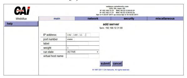
In this screen, you will need to specify the virtual host name of the server you are adding. The WebMux will use this host name when it does the server health check and as the match pattern to direct clients to the correct site.
