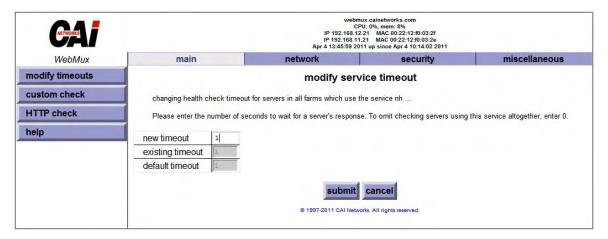
The setting in this page will determine how long or how short the WebMux will wait to be able to verify if the gateway IP is still valid or not. You can disable the checking altogether by setting the timeout value to 0 or you can set the "front network verification" protocol to "none" in the Network Setup page (see Section 6.3).
